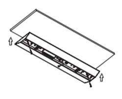
Connect the LED unit and the luminaire body by the safety cable, then connect the power line.
