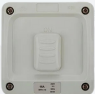
IP66 1 GANG WEATHERPROOF SWITCH 250V 16A 1 POLE 2 WAY
